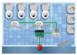
It is recommended that you install your Cig-Arrête System using multi-core stranded alarm cable.
