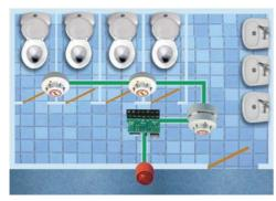
It is recommended that you install your Cig-Arrête System using multi-core stranded alarm cable.
