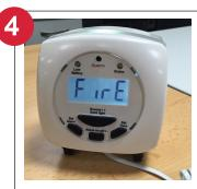
High intensity LEDs will flash and the screen will display "FIRE."
