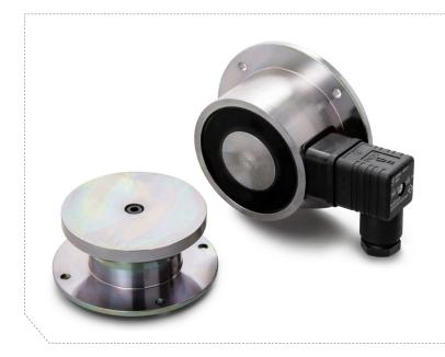
The Weather Proof Door Holder is designed to hold open fire doors for convenient access through busy door ways and release them for closing when an alarm is triggered. It is designed for wall mounting and is supplied complete with a keeper plate for fixing to the fire door. Both parts are constructed from steel and are zinc plated.
