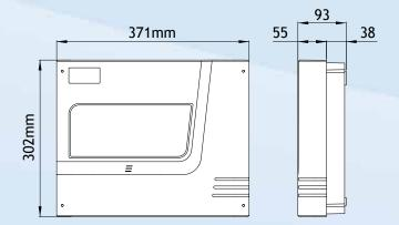
The Infinity 8 control panel is housed in the most attractive, modern designed, flame retardent ABS enclosure, utilising a switch mode power supply. It has a fully removable front cover which improves ease of access for cable installations.
