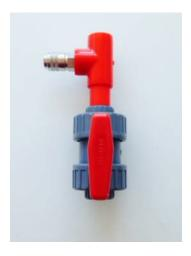
The quick release airline kit is available to suit 25mm or 27mm pipe systems and gives the opportunity to close the system off by turning the ABS ball valve handle to the closed position. Therefore, protecting the aspirator panel from a burst of air introduced at the quick release airline adaptor.
