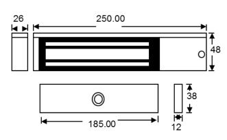
Slim single unmonitored magnetic lock. Compact design, making it ideal for most indoor applications where 275kg holding force is sufficient.
