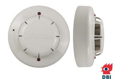
The Fyreye Extra analogue addressable optical smoke detector is particularly suitable for detecting optically dense smoke, involving materials such as soft furnishings, PVC, plastic, foam and all similar materials which produce small visible particles (0.5 to 10 µm).
